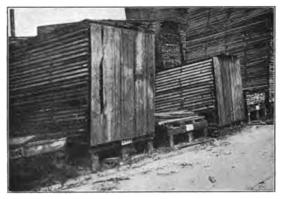
Fig. 88.—Sun shields used to reduce checking in thick red oak timber.
